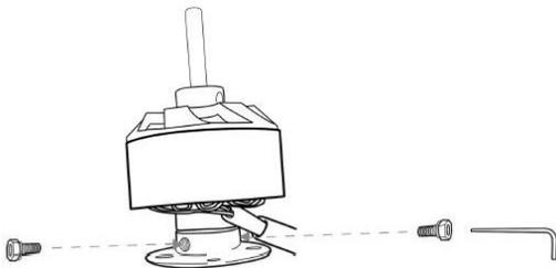
2. Insert the 2812 Motor into the Motor Base.
