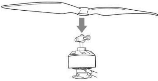
*The Prop Saver is designed to allow the propeller to fold back when it hits the ground. To do this place the Prop Saver towards the tip of the shaft. It shouldn't be too far out that the propeller wobbles when it spins, but not too far back that the prop can't fold back.*
