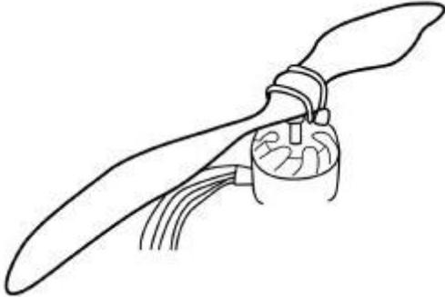
6. Use the Allen Hex Key to put the O-Ring Over the propeller. This will secure the propeller to the 2812 Motor.
