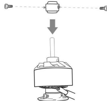
*It is recommended to use a thread locker to keep the screws from loosening themselves due to motor vibration. Check fasteners periodically to make sure they haven't become loose or missing.*
