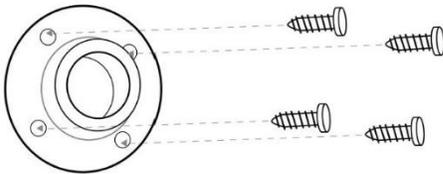
3. (It may be easier to skip to step #4 and do this step last) Use 2x M3 Fasteners and the Allen Hex Key to tighten the 2812 Motor in place. The M3 Fasteners should only be snug. If they are over tightened, the motor wont spin freely and it could damage the bearings beneath.
