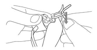
8. Plug in your Motor into a 30A or higher rated ESC.
