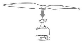
The prop saver is designed to allow the propeller to fold back when it hits the ground, so the motor shaft does not bend. To properly mount the prop saver, place it towards the tip of the shaft. The prop saver should not be too far out that the propeller wobbles when it spins, but not too far back that the prop cannot fold back.
