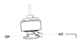
It is recommended to use a thread locker to keep the screws from loosening themselves due to motor vibration. Check fasteners periodically to make sure they have not become loose or missing.
