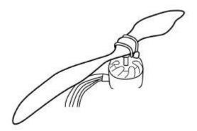
6. Use the Phillips screwdriver to put the O-Ring Over the propeller. This will secure the propeller to the 2812 Motor.
